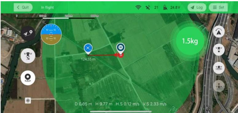
**Notice** the real-time weight values might deviate due to wind and when the SharkX carries no payload, there is no weight display on the flight interface
