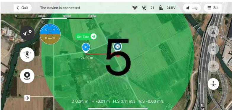
**Notice** the 5-second countdown and the short wait allow users a limited time to finally ensure there are no obstacles around the drone and the fishing line is unlocked on the reel. To avoid any accidents, please make sure the preflight check gets done before starting every mission.
